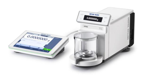
Above: XPR microbalances deliver highest precision (0.1 µg) at lowest minimum weights (30 µg), for fully traceable results, even under challenging conditions. Space-saving design and second terminal are ideal for use in a safety cabinet. Touch-free operation and easy cleaning enable safer weighing. User guidance, built-in results notepad, customized method library and direct data transfer via LabX save time and provide process security.
